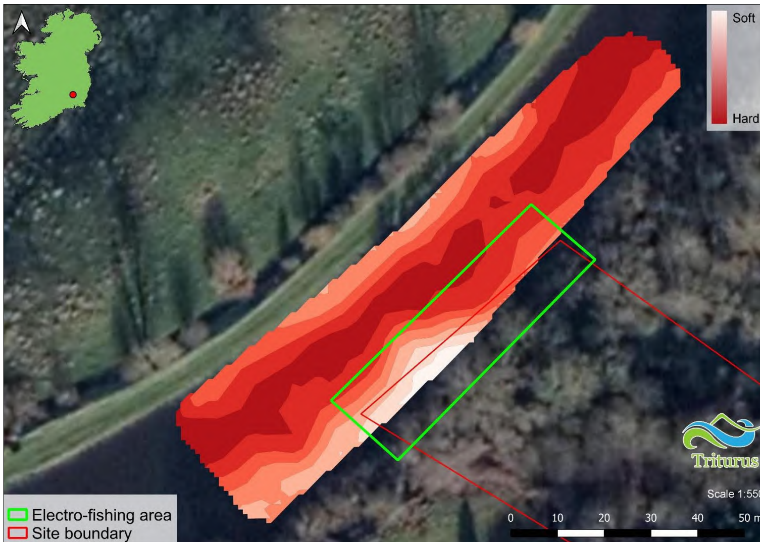
Figure 3.4 Bottom hardness map of the proposed Mortarstown WWTP outfall works area, July 2021 (lighter shading indicates softer substrata)
